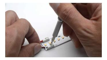
Step 5: Gently tug on the wires to ensure that the wires have been securely inserted and clamped.
