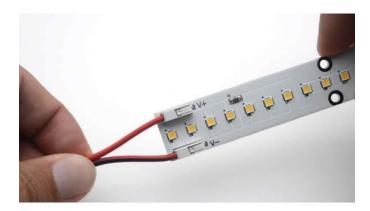
**Step 6:** Plug the DC power plug into the jack, and the DC power supply into a wall outlet. The module should now illuminate.
