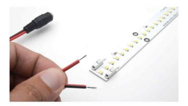
**Step 3:** First, locate the terminal block marked (V+). Then, press down on the terminal block clamp using the dedicated clamp release tool (recommended) or a screwdriver, and while continuing to press down on the clamp, insert the positive (red) wire into the receptacle. Once inserted, let go of the clamp. The wire should now be securely clamped down.
